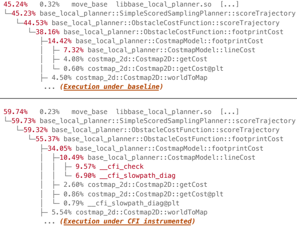
Figure 5: CFI checks extend the worst-case execution paths.
